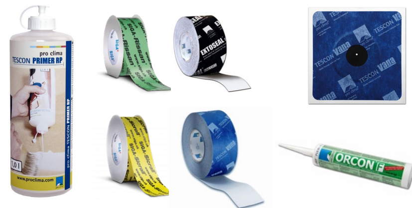
Components of the airtight layer are primarily connected together with tapes. Appropriate primers should be applied to certain surfaces before taping to ensure adhesion. Airtightness grommets and specialised long-life sealants are also available to assist with more specialist junctions in construction. (Sources: Pro Clima, Siga)
